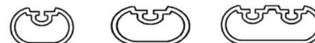
Polished and Bright Dipped Oval Tube (w/ Slot for Insert) left to right: 25-BD-250, 25-BD-255, 25-BD-212
