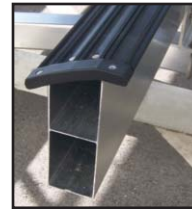
Bunk Bracket, Bunk and Bunk Pad
