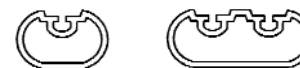
Polished and Bright Dipped (w/ Slot for Insert) single: left; double: right
